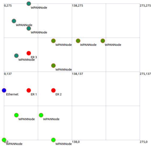
Fig. 2. Sample hybrid network with WPAN, Wi-Fi and CSMA modules
